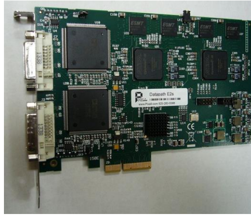
A PCIe 2-port HDMI video capture card (Datapath VisionRGB-E2s)
