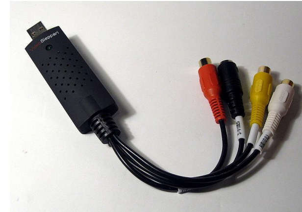
Consumer-grade USB audio/video capture device (Reddo Videosieppari)
